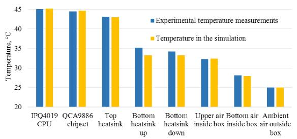
Fig. 5. Simulation and experimental measurement heating temperature comparison
