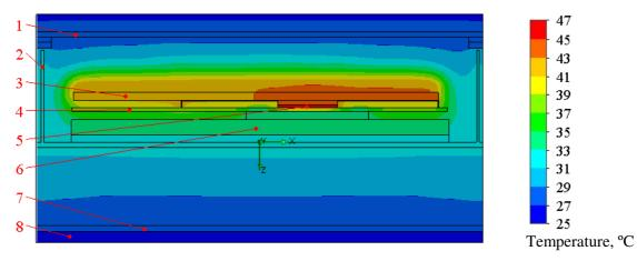
Fig. 6. Temperature distribution of IPQ4019 CPU: 1 -cover; 2 - electromagnetic shield strip;
