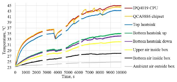
Fig. 4. Experimental temperature measurements using thermocouples
