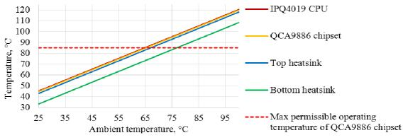
Fig. 8. Simulated component temperature dependence on ambient temperature
