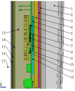
Fig. 1. Structure of the simulation model: 1 – ABS plastic shell; 2 – aluminium sheet; 3 – MS polymer; 4 – solid bottom heatsink; 5 – bottom thermal pad forIPQ4019 CPU; 6 – printed circuit board; 7 – IPQ4019 CPU; 8 – top thermal pad for IPQ4019 CPU; 9 – top heatsink with fins; 10 – QCA9886 chipset; 11 – top thermal pad for QCA9886 chipset; 12 – bottom thermal pad for QCA9886 chipset and resistors; 13 – electromagnetic shield strip; 14 – aluminium sheet; 15 – gasket; 16 – cover; 17 – ambient air
