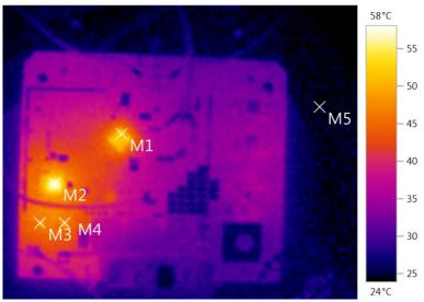
Fig. 2. Thermographic image of PCB without heatsinks
