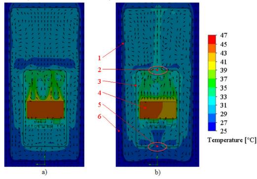
Fig. 3.Airflow trajectory and temperature: a – before electromagnetic shield modification; b – after electromagnetic shield modification; 1 – ABS plastic shell; 2 – top hole in electromagnetic shield;
